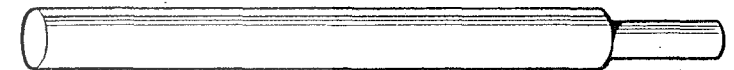
Shoulder Drift for Removing and Fitting Valve Guides. Total Length, 6ins.; Small Diameter, 1in. long; Diameters, 1/2in. and 19/64in.
