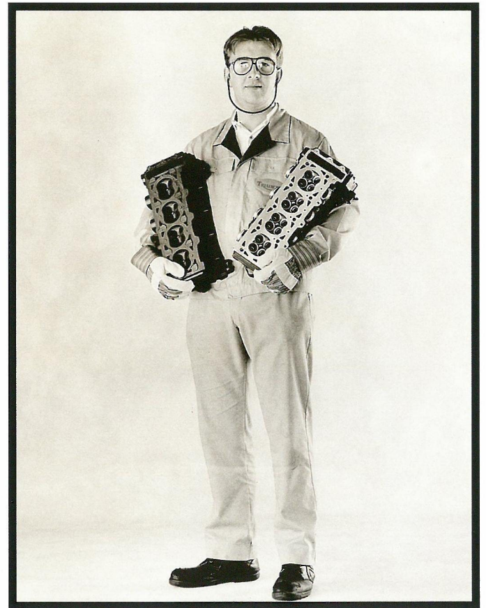
From raw engine castings, it takes 12 separate machining processes at Triumph to transform them into a work of art.
