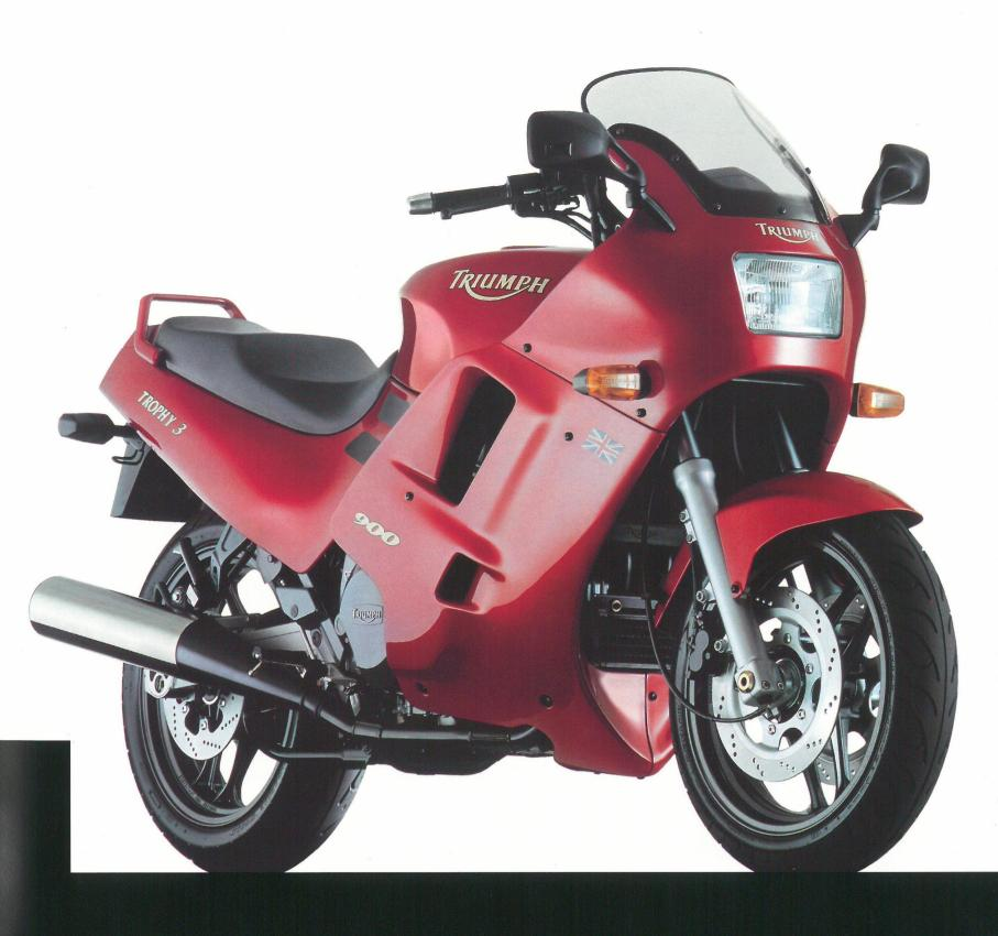
The Trophy now has even better high speed stability thanks to the revised and lowered rear suspension. An improved windscreen design deflects more wind pressure from the rider. Brakes on the 1200 are significantly uprated, with 4-piston caliper twin floating front discs, as used on the Triumph Daytona.
