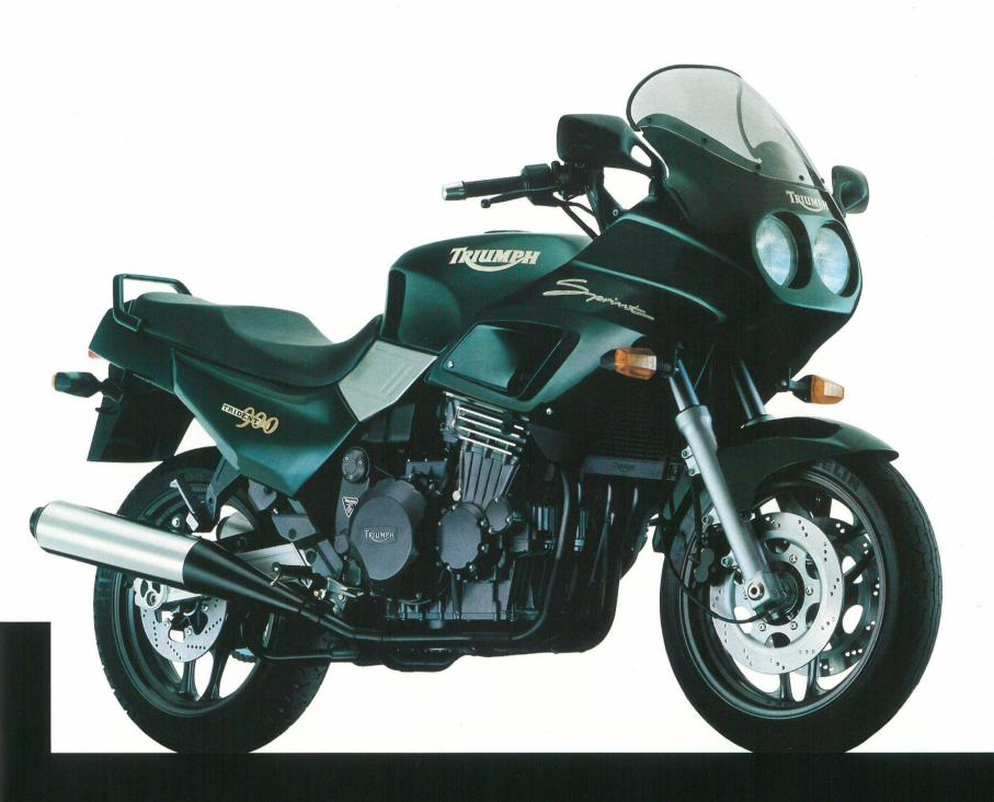
The fairing is fitted with twin quartz halogen headlamps to provide a broader beam of light for night riding. The Sprint shares the unfaired Trident's new lower riding position, and fully adjustable rear suspension from our much acclaimed Trophy model. A choice of colours
