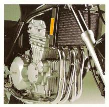
The highly distinctive 12-valve three cylinder engine is fed by a trio of 36mm flat slide Mikuni carburettors. The 120° firing pattern ensures a unique engine note and smooth power delivery that you will never tire of.
