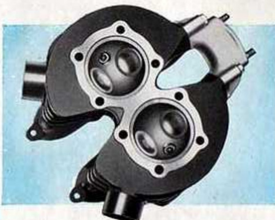
The photographs show (above) the highly efficient hemispherical combustion chambers of the 500 cc. engine. (Left) the 4 gallon petrol tank.
