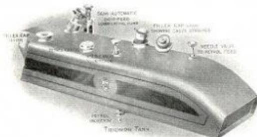
The tank is divided into two compartments, the fore part for lubricating oil, and the rear compartment for petrol. All taps are dispensed with, as they are apt to stick, and needle valves are substituted throughout. Removable strainers are fitted into both the oil and petrol orifices to trap any foreign matter; these orifices are large and have quick detachable caps.
