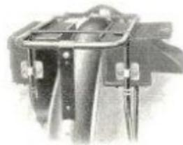
Between the double stays, special brackets or steel shelves are fitted to take the pannier toolbags which are thus protected from mud, and being recessed protrude but little beyond the width of the carrier, and so are of no inconvenience when mounting or dismounting. This leaves the top of the carrier quite free for luggage.
